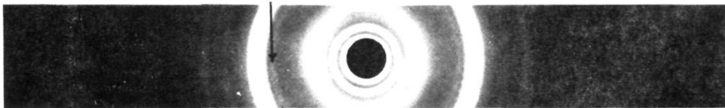
Fig. 7.—Sodium palmitate powder at room temperature cooled rapidly, radius of camera 57.3 mm.
