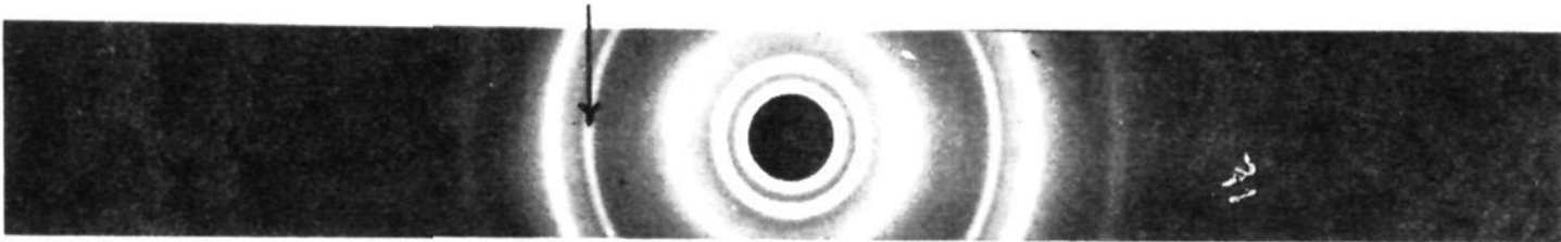
Fig. 6.—Sodium palmitate powder at room temperature cooled slowly, radius of camera 57.3 mm.
